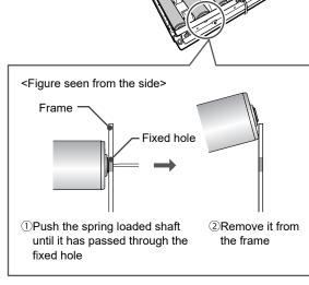
Remove the roller drive belt, and remove the idler
