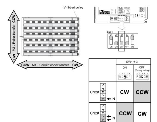
Transfer/Stop in the CW direction \* by inputting signal
