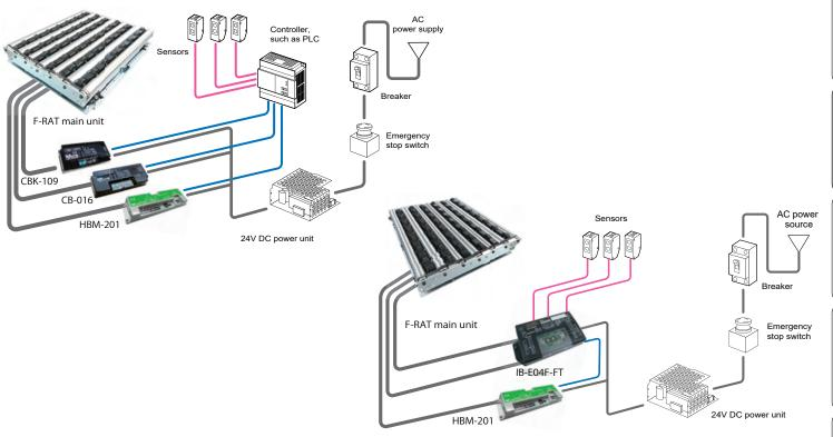
[Important] As for the sensor input, and input/output signals of driver cards, adopt the number of inputs/outputs based on operation.
