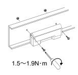
Mounting sensors, control devices, and power supply units
