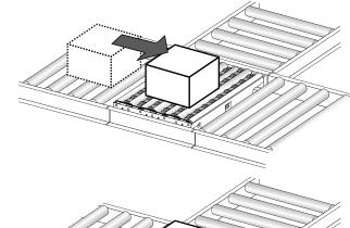
Switch to the diverting direction
