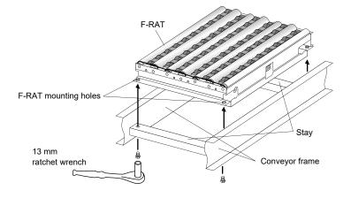
Adjust the conveyor frame legs on which the F-RAT main unit has been mounted, and align levels of the F-RAT main unit and the adjacent conveyor.
