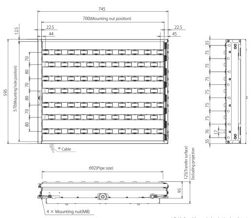
\*Guide for cable marginal projecting length (mm) M1: Carrier wheel transfer MDR 850
