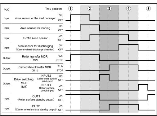
It is assumed that switches on CBK-109 and CB-016 are used based on the initial settings.
