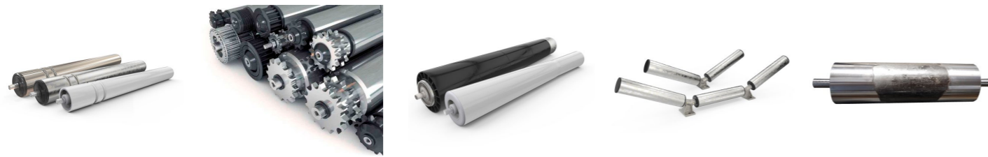
Grooved For band driven and powered roller conveyors. Sprocketed Chain, mini-v, band or tooth belt driven. Tapered For use on bends to guide product around. Troughed To support troughed belt conveyors. Drums Largely used as head and tail drums on belt conveyors.
